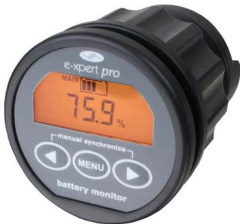
The e-xpert pro selectively displays voltage, charge- and discharge current, consumed amhours, remaining battery capacity and time remaining of your battery bank. Using a clear backlit LC Display and an intuitive user interface, all parameters can be recalled with just a button press. A second battery input is also provided to monitor an auxiliary battery.
